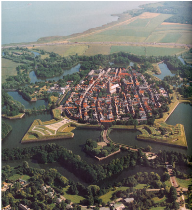
Naarden is the best preserved of the 17 th century fortified towns in the Netherlands. It has a double moat and its bastions are clad with stone. Will, Sterk Water , p. 46.
